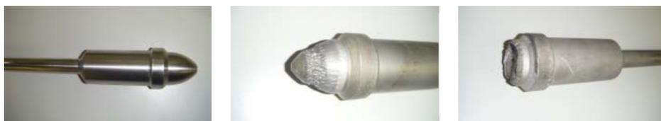
L-R: New plug; Short term wear; Complete failure
