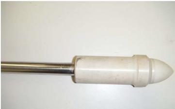
Original plug stem, 2 piece design, 316SST stem with Ceramic tip. Life span of approx 1 – 2 weeks with failure mode being cracking of the ceramics at the threaded connection, likely due to thermal shock.
