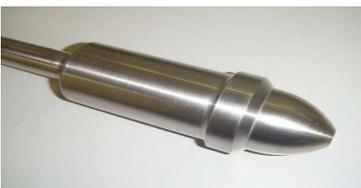
Fourth design, 1 piece 316SST/ COCRA (Alloy 6) plug stem. Four month lifespan with Hardide coating. Now standard fit on all AA valves.
