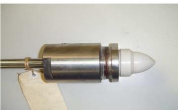
Third design, 316SST stem with retained ceramic tip. This design was to alleviate plug tip wear and ensure positive connection of stem to plug tip. Ceramic tips snapped off due to thermal shock. Lifespan of hours/ days.
