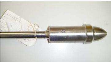
Second design, 2 piece construction 316SST/ COCRA plug with pinned 316SST stem. Failure occurred with wear of plug and separation of plug/ stem likely due to vibration. Lifespan 3-4 weeks.
