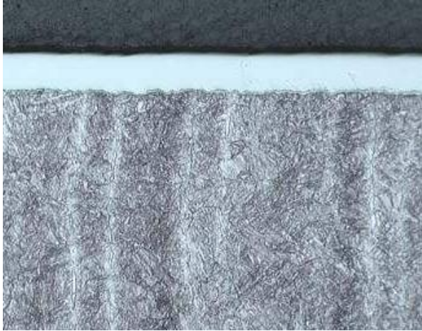
Fig. 7. Pore-free Hardide™ coating protects the substrate against aggressive media attacks; a micrograph of a Hardide-coated sample of 17-4 stainless steel after 30 days in solution of NaCl, Acetic Acid and H 2 S (micro-photograph from Bodycote report [7]).
