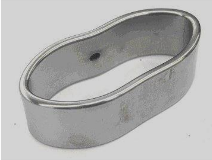
Fig.9. Steel test ring with 50 microns Hardide coating crushed to test coating adhesion and toughness – no flaking or coating separation from substrate
