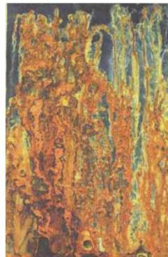
Hard Chrome – had to be removed after 288 hours due to severe corrosion
