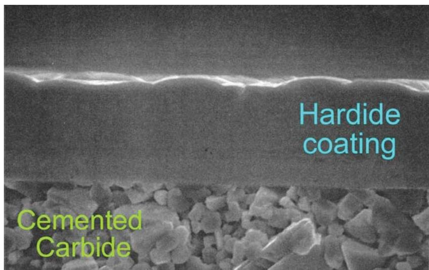
Hardide CVD coating on cemented carbide.
