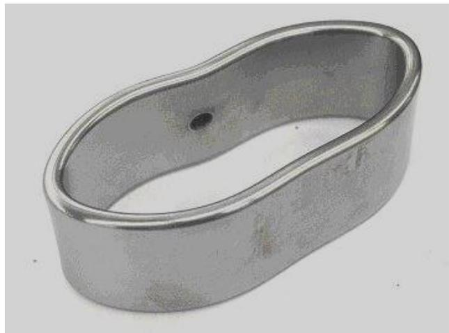
*Fig.3. (Left): Micro-photograph of a crater (diameter approx. 1 mm) made by impact into 50 microns thick Hardide-T coating. Fig.4. (Right) Steel test ring with 50 microns Hardide coating crushed to test coating adhesion and toughness – no flaking or coating separation from substrate*
