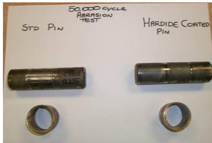
Fig. 4. Rotating pin after 50,000 cycles of abrasion tests in sand/water slurry under high load: the coating reduced pin wear rate by a factor of x70 - as compared to standard case hardened pin. The uncoated brass bushing wear was also cut by a factor of 2.5 thanks to the Hardide coating's non-abrasive properties.
