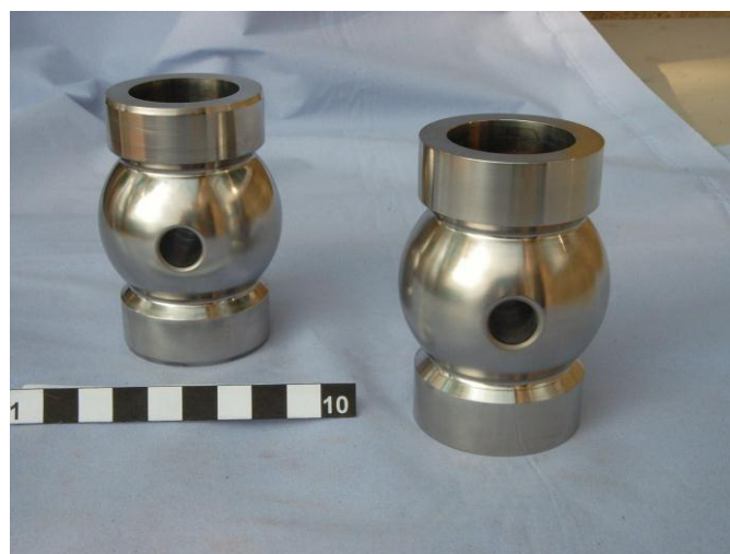
FIGURE 15 - Ball valves coated with CVD Tungsten Carbide coating.
