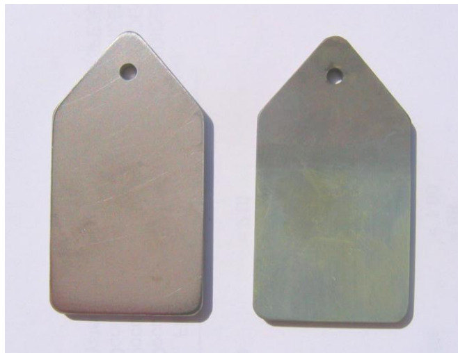
FIGURE 7 - CVD Tungsten Carbide-coated 316 stainless steel samples: untested (left) and tested for 113 hours in 20% Nitric acid (right).
