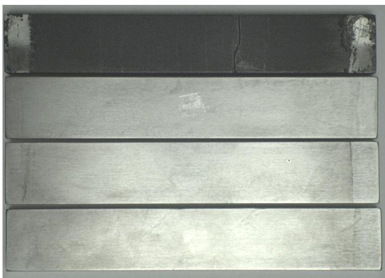
FIGURE 5 - Stressed faces of Uncoated (top) and CVD-coated (N 2, 3 and 4 from the top) samples of 17-4 PH stainless steel after 30 days Sulphide stress cracking test (photo from report 6 ).
