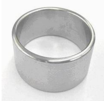
FIGURE 8 - 4140 steel test ring with 50 microns CVD Tungsten Carbide coating type T after 24-hours immersion in uninhibited 28% HCl – no appearance change or weight loss were detected.
