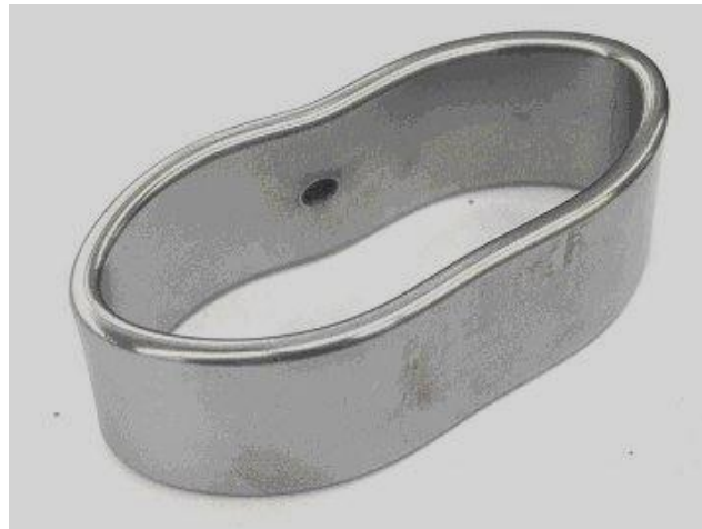
FIGURE 12 - Steel test ring with 50 microns CVD Tungsten Carbide coating crushed to test coating adhesion and toughness – no flaking or coating separation from substrate
